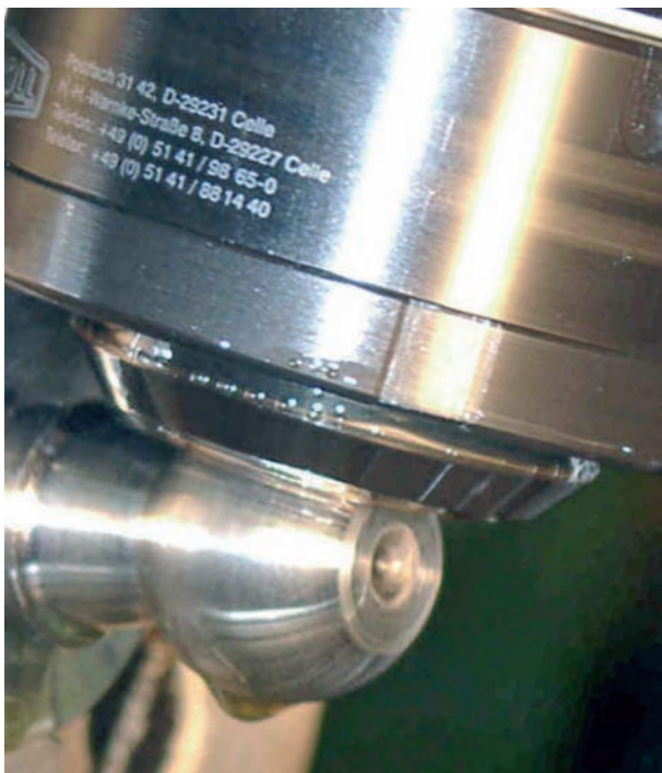
RKAK tool in operation
