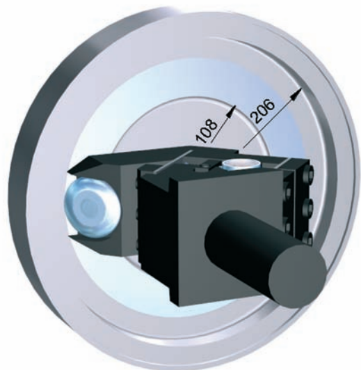
Machining a flywheel with an EG45-40M tool.
