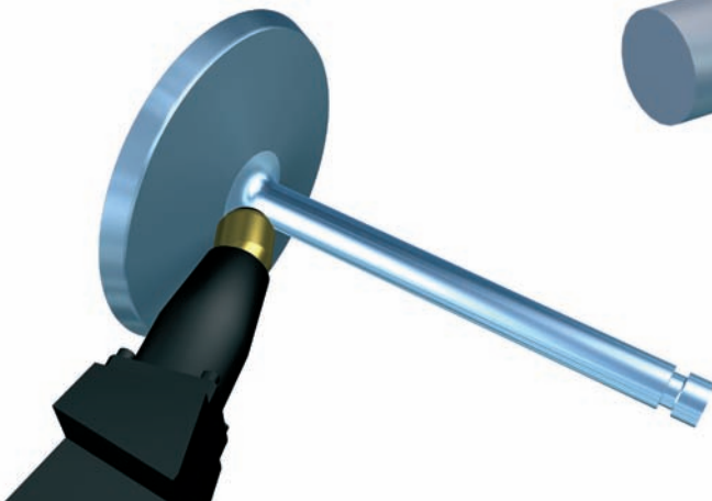
Deep rolling a valve with an HG6 tool to improve its fatigue strength.
