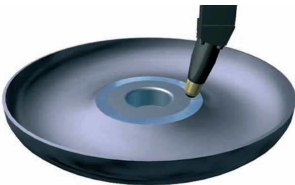
Roller burnishing a torque converter housing with an HG13 tool to improve its sliding properties.
