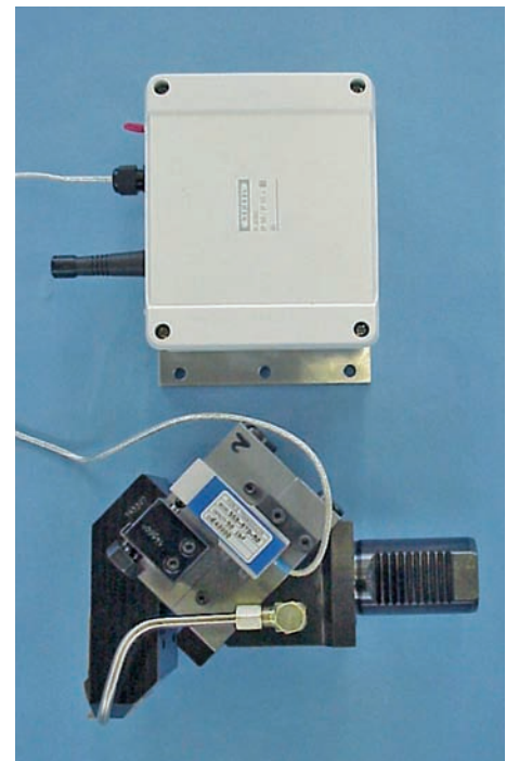
Connecting the transmitter to the deep rolling tool
