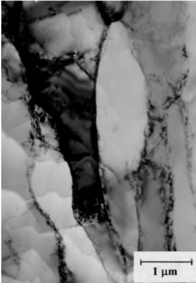
Fig. 11 Near surface ( z = 0.12 mm) dislocation distribution in shot-peened AlMg1. Shot size S170, 54-58 HRC, p = 0.24 bar, coverage 98%
