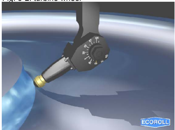
Fig. 5-3: deep rolling turbine wheel with HG13
