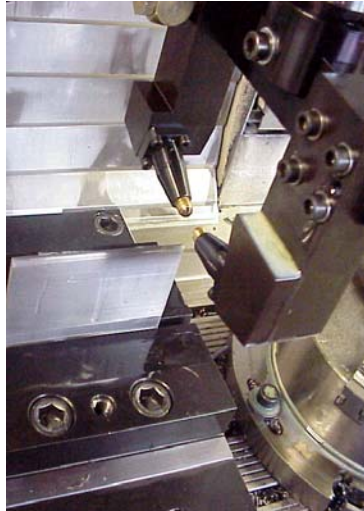
Fig.5-5: deep rolling of turbine blades in longitudinal direction
