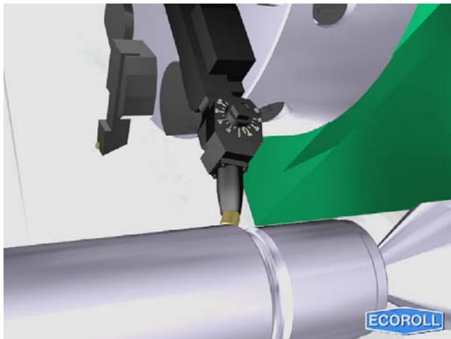
Fig. 10-1: deep rolling of a screw thread undercut
