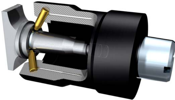
Fig. 7-8: rotating deep rolling tool
