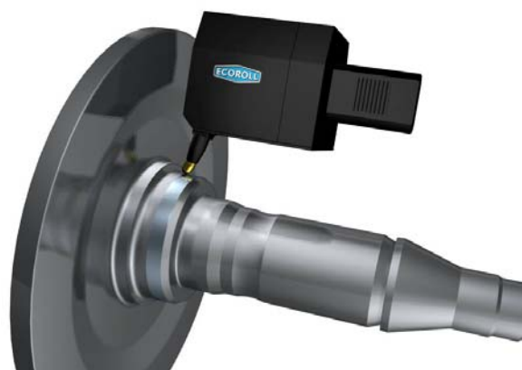
Fig. 7-10: deep rolling of driven rear axles
