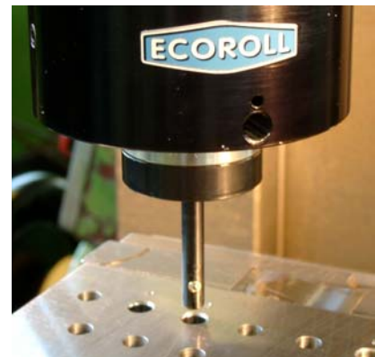
Fig. 12-3: deep rolling of bolt holes
