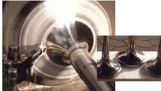
Fig. 4-1: deep rolling of valves for diesel engines
